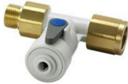
John Guest Angle Stop Valves are manufactured in Acetal with EPDM 'O' Rings. They incorporate a single check valve and a 1/4 turn chromium plated ball valve. The valves are for use with potable water.
