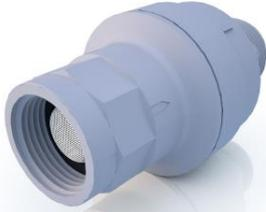
The Water Block valve is an overflow safety device, which controls the maximum consumption of water between 5 and 50 litres. If this quantity exceeds the set value, the Water Block stops the flow and keeps this safety condition until user intervention.
